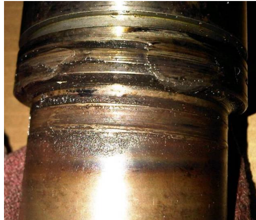
Damaged oil return threads
