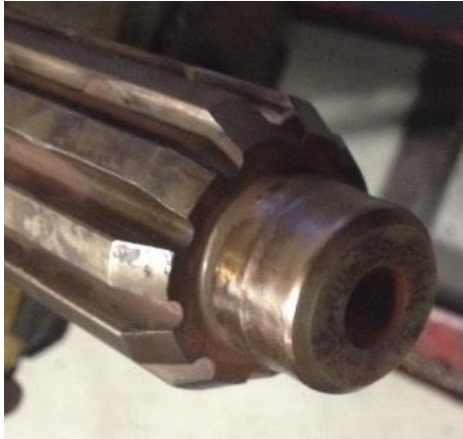
Worn input shaft pilot surface
